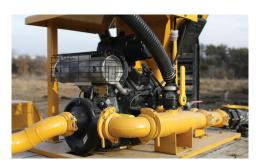
POWERFUL PERFORMANCE. The MX300 is equipped with a 23 hp (17.2 kW) Kohler ECH 730 EFI engine and 350 gpm (1324.9 Lpm) pump flow to help provide powerful performance to the job.
