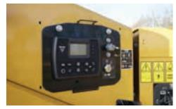
**ECOIDLE<sup>TM</sup> ENGINE CONTROL SYSTEM.** When the Ecoldle system is selected by the operator, the engine speed automatically lowers to a preset rpm after one minute or five minutes of inactivity to help reduce fuel consumption when not chipping material. This idling can help reduce emissions and noise.
