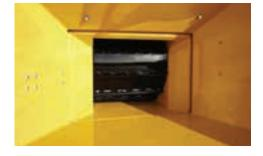
**FEED ROLLER.** A large letterbox infeed opening at 44 cm x 30 cm helps boost productivity by reducing the need to trim material before feeding it into the chipper.
