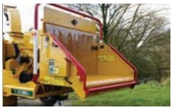
**SMARTFEED.** The SmartFeed system monitors engine rpm and automatically stops and reverses the feed roller to maximize productivity. This system also senses feed roller jams and manipulates the material automatically to reduce the need for manual control bar use.
