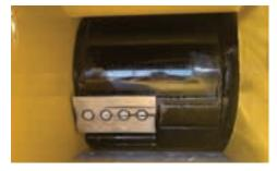
**CHIP DRUM.** The Vermeer BC1000XL brush chipper uses a precision-balanced drum with two A8 double-sided knives to chip through material up to 30 cm in diameter.
