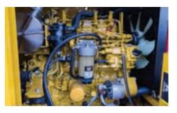
**POWERFUL PERFORMANCE.** The 74 hp (55 kW) Stage V compliant Caterpillar diesel engine allows you not only to comply with Stage V emissions requirements, but also gives you the engine power to meet your jobsite needs.
