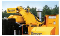
REPLACEABLE WEAR PARTS. High-wear material flow areas of the machine, such as the drum, discharge chute, cutter housing and infeed conveyor floor, are designed with replaceable bolt-in wear parts to extend machine life.
