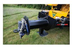
JOBSITE MOBILITY. The WC2300xL has a compact design and built-in skidder grab on the tongue, allowing it to be moved around on the jobsite by a skidder or excavator.
