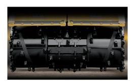
**TERRAIN LEVELER® SURFACE EXCAVATION** MACHINE (SEM) ATTACHMENT. The T9555III has a chain drive Terrain Leveler SEM optional attachment for large rock excavation applications including surface mining, overburden removal, site preparation and road demolition.
