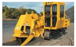
HYDROSTATIC ROCKWHEEL ATTACHMENT. Powered by a hydrostatic motor, the rockwheel attachment has the ability to cut a trench up to 36" (91.4 cm) in depth and 6" (15.2 cm) in width.
