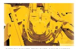
ROTARY POWER TRENCHER DRIVE MOTOR. A rotary power trencher drive motor and splined headshaft produce a lower speed and higher
