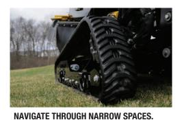
When you need to navigate through narrow iobsites, you can retract the machine to only 35 in (89 cm) and then extend the tracks to 49 in (124.5 cm). The tracks are low disturbance, and they provide optimal traction and stability in tough ground conditions-leaving you with minimal job prep and clean up afterwards.
