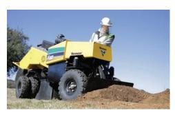
**OPTIONAL HYDRAULIC PUSH BLADE.** The optional hydraulic push blade on the SC382 simplifies jobsite cleanup by helping maneuver processed material.
