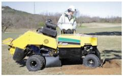
STANDARD FOUR WHEEL DRIVE. Four-wheel drive comes standard on the SC382. It offers traction and maneuverability in difficult transport conditions.
