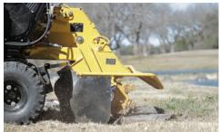
ROBUST CUTTING POWER. The SC382 is equipped with a 37 hp (27.6 kW) Briggs and Stratton Vanguard engine, giving you power straight to the stump.
