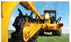
**MAXIMUM PRODUCTIVITY.** The dedicated plow has a maximum installation depth of 24" (61 cm), while the optional trencher attachment has a maximum trenching depth of 42" (106.7 cm) and width of 6" (15.2 cm).
