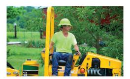
JOBSITE VISIBILITY. The operator seat sits at the center of the service plow directly above the machine's articulation point, which provides excellent visibility of the entire work area.
