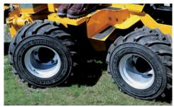
ARTICULATED DESIGN. The center-articulated PTX44 oscillates at the point of articulation, providing unmatched performance on uneven terrain.
