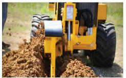
MACHINE VERSATILITY. Utilized for irrigation and utility installations, the versatile PTX40 is a plow/trencher with a dedicated plow depth of up to 24" (61 cm), a trench depth of up to 42" (106.7 cm) and a width of 4-6" (10.2-15.2 cm). The optional bore attachment has a maximum torque of 494 ft-lb (670 Nm).
