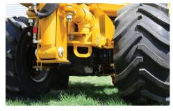
TRACTION OPTIONS. With a variety of different traction options, the PTX40 is well-suited to contractors' differing needs. The 23" (58.4 cm) tire option is best for narrow, congested jobsites, the 26" (66 cm) tire option provides better traction, and the dual tire option accommodates lower ground pressure requirements. Additionally, the PTX40 is available with tracks which are ideal for uneven terrain.
