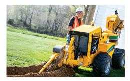
COMPACT SIZE. At 40.2" (102.1 cm) wide and only 55" (139.7 cm) high, the PTX40 is small enough to navigate smaller jobsites where larger machines can't fit.
