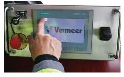
**CONTROL AT YOUR FINGERTIPS.** A tethered human-machine interface (HMI) with user-friendly touch screen allows the operator to monitor and set all the parameters of the pump from remote.
