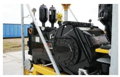
**FLOW RATE AND POWER.** A fully electric high-pressure mud pump capable of delivering an adequate flow rate for large pipeline installation by horizontal directional drilling. The powerful electric 339-kW Danfoss motor drives the Tecniwell TW2500 HDD triplex piston pump, which is the core of the system, making this pump the ideal match with maxi rigs.
