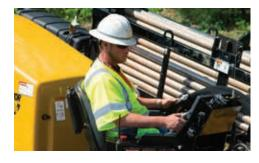
SIGNIFICANT SOUND REDUCTION. With a 104 dB(A) guaranteed sound power level and an operator ear rating of 82.9 dB(A), as well as an in-cab operator ear rating of 75.7 dB(A), the D24x40 S3 contributes to a quieter working environment, creating less neighborhood disturbance and enabling easier communication among the crew.
