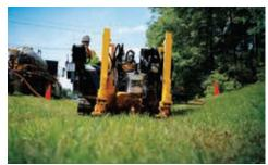
WHEN THERE'S A JOB TO BE DONE. With 28,000 lb (124.6 kN) of thrust/pullback and 4200 ft-lb (5694.4 Nm) of rotational torque, the D24x40 S3 offers an increase over its predecessor, helping to maximize machine and jobsite productivity.
