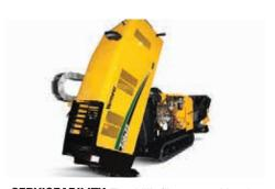
SERVICEABILITY. The drill's flip-up metal hood offers ease of access when performing routine service and maintenance.
