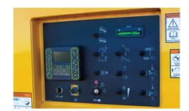
CONTROL SYSTEM. Operators can control the machine through either the Vermeer DP10 display mounted on the control panel, or through a hand-held transceiver remote. From either control, the operator can choose from four programmable presets or adjust on the fly based on the incoming material.
