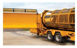
DRUM SERVICE ACCESS. A single-hinged side panel exposes the full length of the trommel drum from ground level for drum service and removal.
