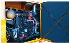
ENGINE. The TR620 features a Cummins QSB 3.3l Tier 4i (Stage IIIB), 120 hp (90kW) engine. The engine is mounted on a pivoting frame that swings out 30 degrees for superior access to fuel filters and hydraulic reservoir for maintenance and service.
