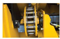
DRUM DRIVE. A hydraulic chain drive system allows the drum to lift off the cog for service. Bolton sprockets can be changed quickly and help lower repair costs.
