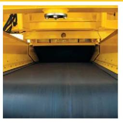
Undermill conveyor. A smooth, 60" (152 cm) belt enables high-volume product removal. To resist tear and puncture, the conveyor is constructed of .5" (1.3 cm) thick rubber belt.
