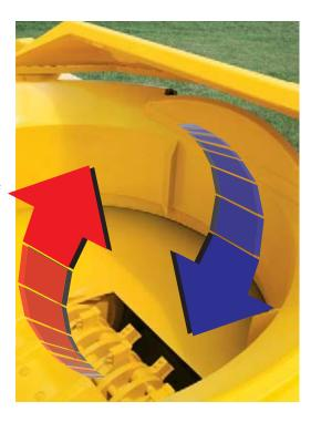
Thrown Object Restraint System (TORS). The patented conical TORS has a smooth underside for increased life and better material flow while reducing the quantity and distance of thrown objects when positioned above the tub.
