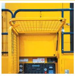
**Fallen Object Canopy.** For enhanced operator safety, the Fallen Object Canopy helps protect operators from falling debris while positioned at the control panel.
