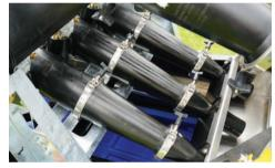
**CLEANING EFFICIENCY.** Premium cleaning performance is achieved through six 4-in long-body hydrocyclones in combination with a relatively large screen area.
