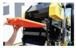
**QUICK-CHANGE SCREENS.** The primary screens are kept in place with an air-clamping system, powered by an onboard air compressor. This allows for ease of access and the ability to quickly change the screens.
